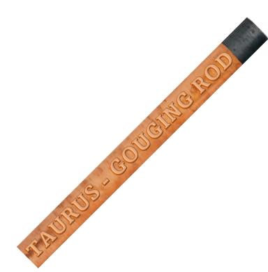
TAURUS gouging carbon, also known as air-carbon arc cutting, is a metal removal process utilising the heat generated by an arc between a carbon electrode and the workpiece. Compressed air, directed through outlets on the torch, lifts molten metal away from the arc, preventing it from solidifying and consequently facilitating metal removal smoothly. Common applications are for weld-metal removal, backgouging and reshaping torn metal.
