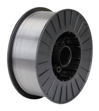
TAURUS E71T is a rutile-type, mixed gas(75% argon / 25% CO<sub>2</sub>) shielded flux-cored wire for welding carbon manganese steels. It is recommended for the all positional welding of mild and low-alloy steels with a tensile strength of up to 620 MPa for general purpose fabrication. This wire provides increased toughness at sub zero temperatures. It has low spatter levels and the slag is easily removable.
