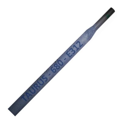
TAURUS PRO INOX 680 is a rutile, austenitic-ferritic coated electrode with 25-30 % ferrite content. The weld metal is extremely crack resistant and lends itself admirably to the welding of dissimilar and difficult-to-weld steels. It can be used for the welding of high-nickel alloys without becoming fully austenitic due to nickel pickup.
