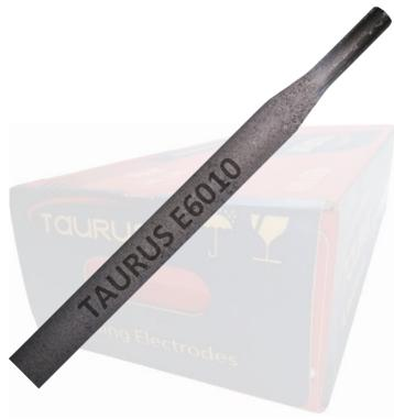
TAURUS PRO 6010 is a medium coated, DC, cellulosic electrode for welding vertical down in pipeline and storage tank construction. Recommended for root-filler layers in pipeline applications. An extremely fast deposition rate can be obtained applying a touch or short-arc technique. The electrode provides a very steady arc over a wide range of current
