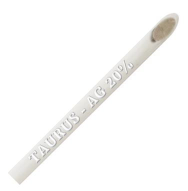
Our TAURUS SILVER SOLDER 20% which is cadmium free and is suitable for use on all ferrous and non-ferrous metals, except aluminium. It can be used with a range of heat sources and is available in bare and flux coated and in various percentages of silver. Our flux coated silver solder has a special fast-flow flux which improves base metal cleansing action.
