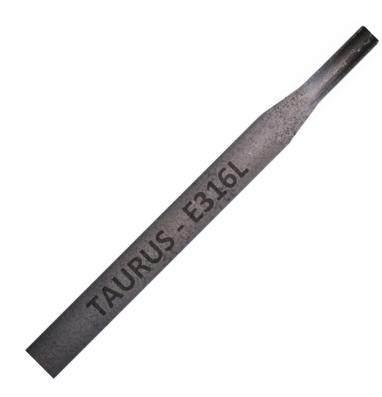
TAURUS PRO 316L is a rutile, high-alloy, extra-low carbon austenitic electrode for welding corrosion resistant CrNiMo steels resistant to atmospheric corrosion. Resistant to grain disintegration at operating temperatures up to 350°C. Very smooth weld with clean weld edge, low spatter loss and easy slag removal. Suitable for welding AISI/ASTM 316, 316L, 316LN, 316H and 316Ti.
