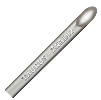
The Taurus ZN-AL02 is a flux cored zinc-aluminum brazing alloy that has a low brazing temperature with a good welding effect. It is used for brazing aluminum to aluminum, aluminum to copper and aluminum to stainless steel. The low brazing temperature makes brazing thinner material easier. Due to the flux-core there is no need for extra flux when brazing. Its main usages are in the field of heat-exchangers ,air conditioners and condensers and automotive refrigeration systems.
