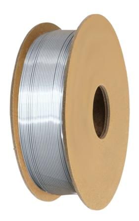
The Taurus MIG 4047F is an aluminium alloy wire with a high silicon content of approximately 12%. The high silicon content ensures a low melting point and excellent fluidity which is ideal for brazing.
