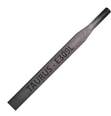
TAURUS PRO 309L is a rutile, extra-low carbon-resistant electrode for welding corrosion resistant and heat resistant CR and CrNi steels. The high level of alloying elements also makes this electrode suitable for welding Cr and CrNi steel to mild steel. Very smooth weld with clean edge, low spatter loss and excellent slag removability.
