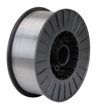
The TAURUS PRO MIG Ni99 wire is a nickel-based welding wire extensively employed to repair grey iron castings as well as for joining cast irons to mild steels and stainless steels. It can also be used for overlay and buildup. A preheat and inter-pass temperature of 175°C minimum is recommended during welding. It offers good weldability, strong, dense weld deposits and is fully machinable. Mixed shielding gas required is 75% argon/25% helium.
