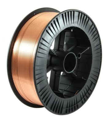
TAURUS MIG SILICON BRONZE is a pure copper filler wire deoxidised with 3% silicon for welding a wide range of copper alloys including overlaying of steels and cast irons. The wire is optimised for laser brazing.
