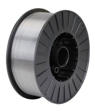
TAURUS E71T-1 is a rutile type CO2 shielded flux-cored wire for welding carbon-manganese steels. It is recommended for the all positional welding of mild and low-alloy steels with a tensile strength of up to 620 MPa for general purpose fabrication. This wire provides increased toughness at sub zero temperatures.
