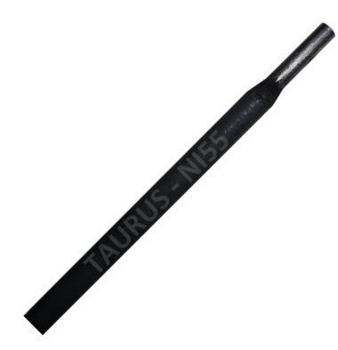
TAURUS PRO Ni 55 is an all positional electrode depositing a 55% Ni/45 % Fe weld metal designed specially for strength welding of grey cast iron and malleable cast iron with steel. Also designed to operate at low current which minimises heat input and thus facilitates the cold welding of cast iron. Weld induced stresses can be reduced by hammer peening. Stable arc with clean bead appearance. The weld metal is fully machinable.
