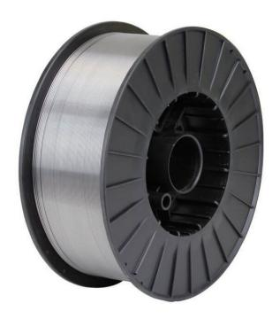
TAURUS MIG 310 wire has good oxidation resistance at high temperatures due to its high content of Chromium. The alloy is widely used for welding heat resistant austenitic steels of the 25% Chromium and 20% Nickel types and therefore sensitive to hot cracking. Common applications are industrial furnaces and boiler parts as well as heat exchangers.
