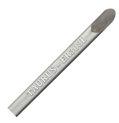
TAURUS TIG 308L rod is used for welding 18/8 stainless steels including 301, 302, 303, nitrogen-bearing 304LN and similar. Service temperatures are typically -100°C to approximately 400°C.
