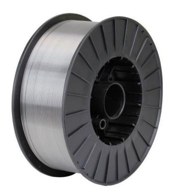
TAURUS ER70S-6 copper-free, mild steel is a premium quality MIG wire produced from high-quality de-oxidised rod. It features good feed ability, extended torch-tip life for improved productivity and good electrical conductivity and reduced friction during high-speed welding. Suitable for butt and fillet welding in all positions.
