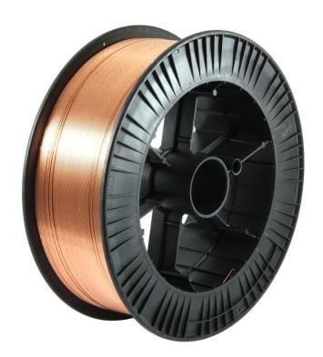
TAURUS MIG WIRE ER100S-G is a low-alloy steel welding wire containing nickel, molybdenum and vanadium. The wire, which is copper coated, is suitable for use in all positions. TAURUS MIG WIRE ER100S-G is recommended for welding a range of fine grained structural steels and low-alloy quenched and tempered steels having an ultimate tensile strength of up to 930 MPa. Argon based shielding gases are recommended.
