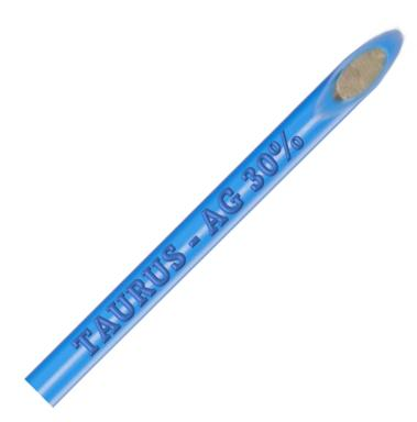
Our TAURUS SILVER SOLDER 30% which is cadmium free and is suitable for use on all ferrous and non-ferrous metals, except aluminium. It can be used with a range of heat sources and is available in bare and flux coated and in various percentages of silver. Our flux coated silver solder has a special fast-flow flux which improves base metal cleansing action.
