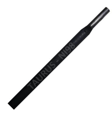
TAURUS PRO Ni 98 is a pure nickel electrode which is universally used for welding all types of cast iron. Specially designed to operate at low currents which minimises heat input and thus facilitates the cold welding of cast iron. Weldinduced stresses can be reduced by hammer peening. Stable arc with clean bead appearance. The weld metal is fully machinable.
