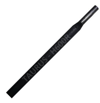
TAURUS PRO H600R is a rutile-coated, hard-facing electrode for surfacing worn parts of civil engineering, construction and mining machinery to be used without machining. Deposited metal of approximately 600 HV provides high toughness in spite of high hardness and excellent abrasion resistance to medium impact.
