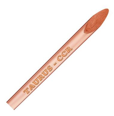
TAURUS Copper Coated Rod (CCR) is a general purpose low carbon steel gas-welding rod which is copper coated to reduce corrosion. It is recommended for oxygen-acetylene welding of mild steel and is widely used in sheet metal work, the heating and ventilation industries, car body repairs, welder training schools and for low pressure piping and plumbing.
