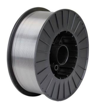
TAURUS MIG 312 wire has good oxidation resistance at high temperatures due to its high content of Chromium. The alloy is widely used for joining dissimilar steels, especially if one of the components is fully austenitic, and for steels that are difficult to weld, like for example machine components, tools and austenitic manganese steels.
