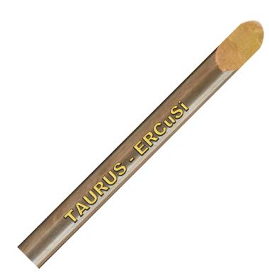
TAURUS TIG SILICON BRONZE is pure copper filler rod deoxodised with 3% silicon for welding a wider range of copper alloys including overlaying of steels and cast irons. TAURUS TIG SILICON BRONZE should be shielded with pure argon but pure helium provides deeper penetration, higher travel speeds and allows reduced preheating.
