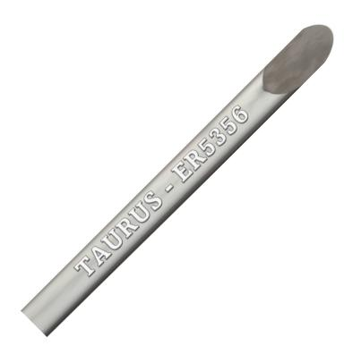
TAURUS TIG 5356 is a 95% aluminium, 5% magnesium rod for general purpose welding when 40 000 psi tensile strength is not required. TAURUS TIG 5356 should be used with a zirconated tungsten electrode with pure argon or an argonhelium mixture for thick sections, at a flow rates of 10 - 15 l/min. For oxy-acetylene gas welding, a neutral flame should be used with aluminium welding flux.
